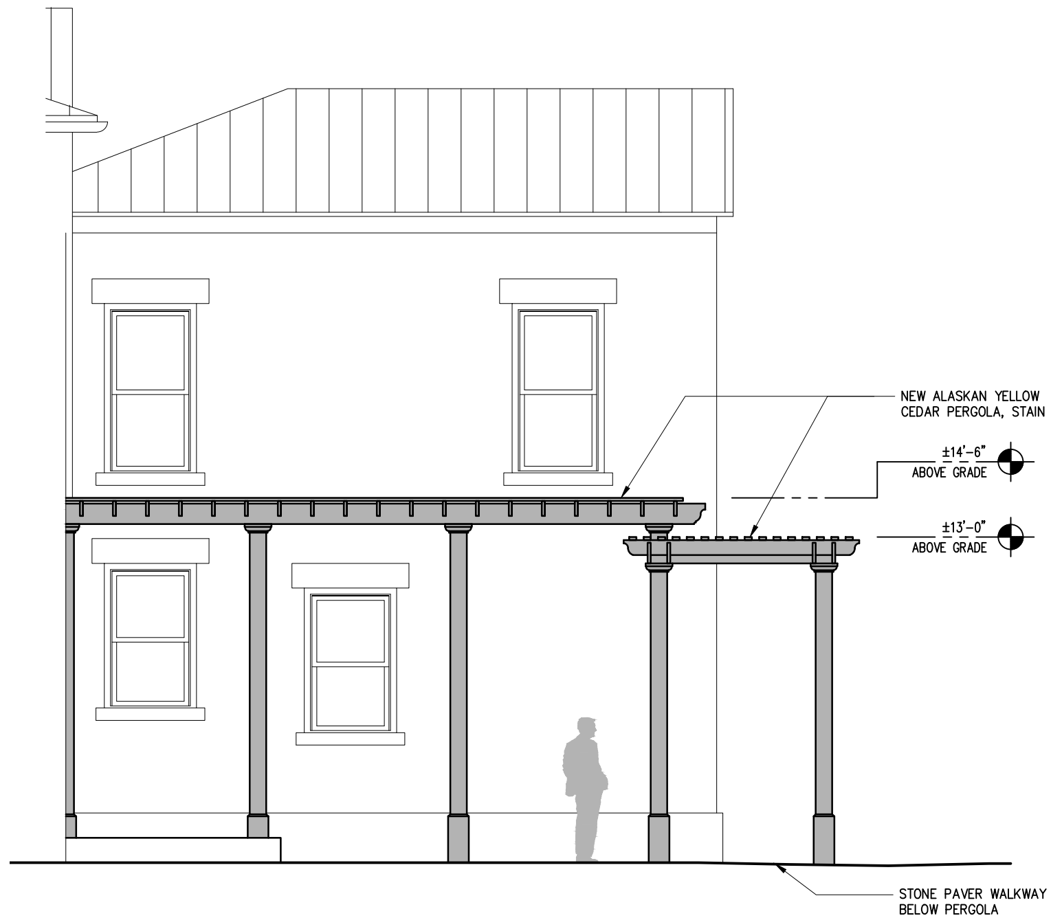
ELEVATION: LEFT SIDE, PROPOSED PERGOLA SCALE: 3/16" = 1'-0"
