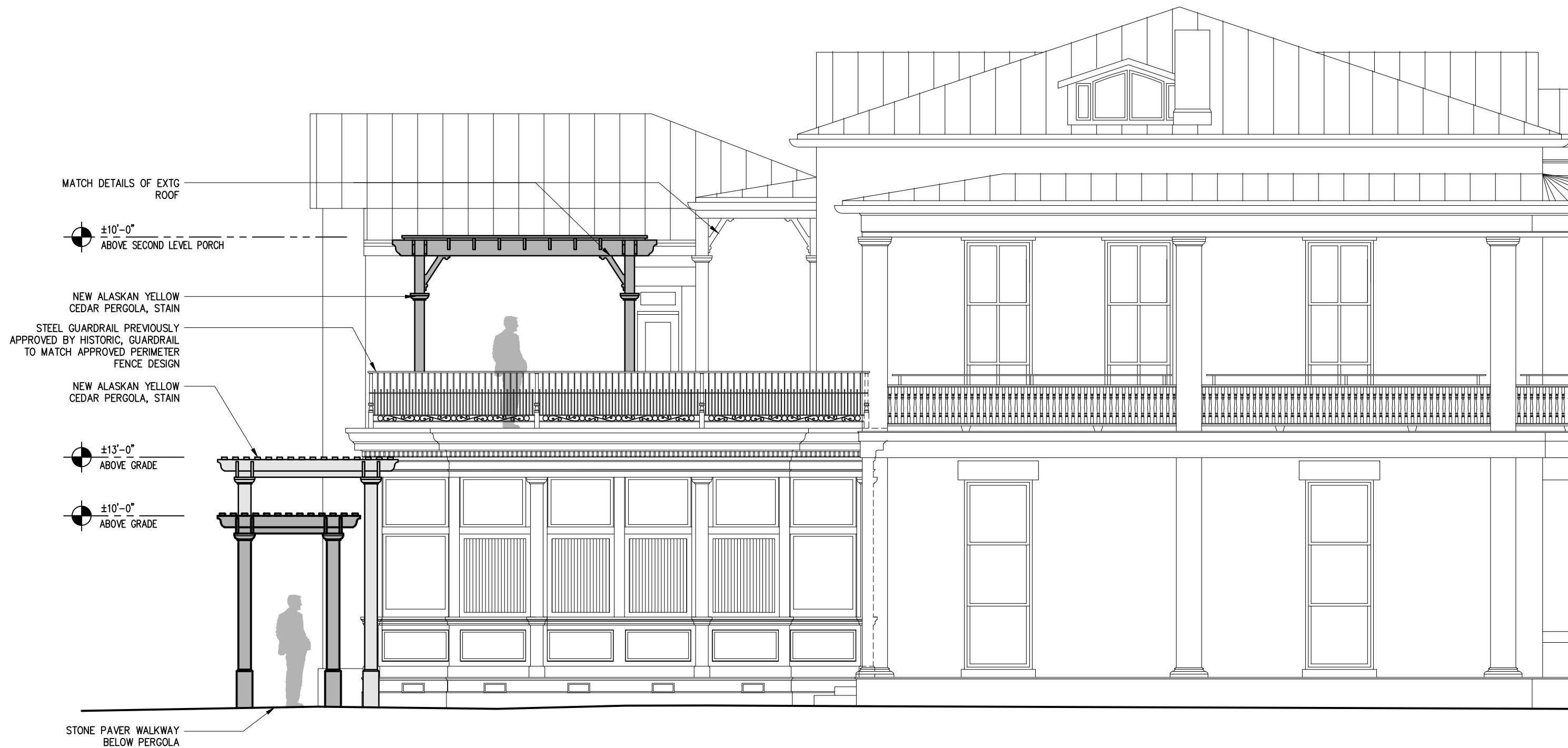
ELEVATION: KING WILLIAM STREET SIDE, PROPOSED PERGOLA SCALE: 3/16" = 1'-0"
